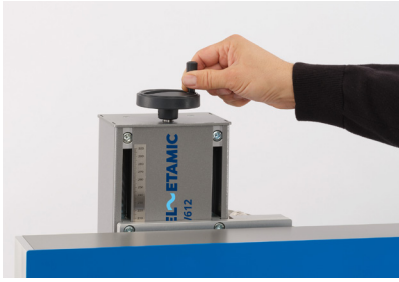
Manual height adjustment for precise probe positioning
