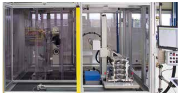
Combined cylinder inspection with CF1250 and B100 sensors
