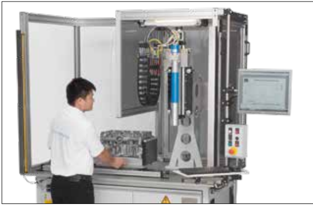
Station with manual loading for small series or prototype production
