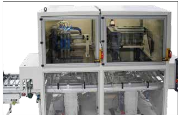
Full inspection of cylinder bore and plane surface on the engine block
