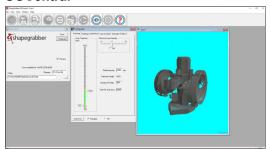
SGCentral is a user-friendly application that lets you configure scan settings, speed, and resolution for ShapeGrabber scanning systems. File formats supported are .gpd (Geomagic), .psl (Polyworks), .stl, xyz (ASCII generic), and others. SGCentral is included with every ShapeGrabber system.
