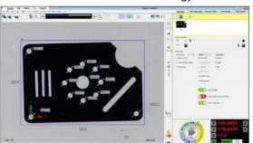
SNAP-X software provides users with a simple, powerful interface for instant 2D measurement and auto program generation. The software also utilizes powerful GD&T based algorithms and point and click feature identification to easily program a wide variety of parts. Virtual chart gaging, profile analysis tools and integrated reporting allow for quick and easy output of measurements.
