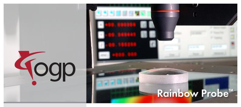
**Rainbow Probe** is a non-contact chromatic confocal sensor that measures surfaces by analyzing changes in the optical spectrum as a function of part to probe spacing. Additional capabilities include:
