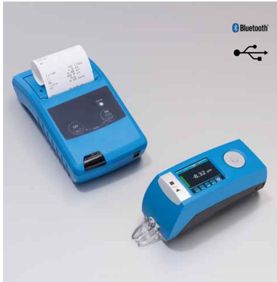
Waveline W5 with optional printer Waveline P5
