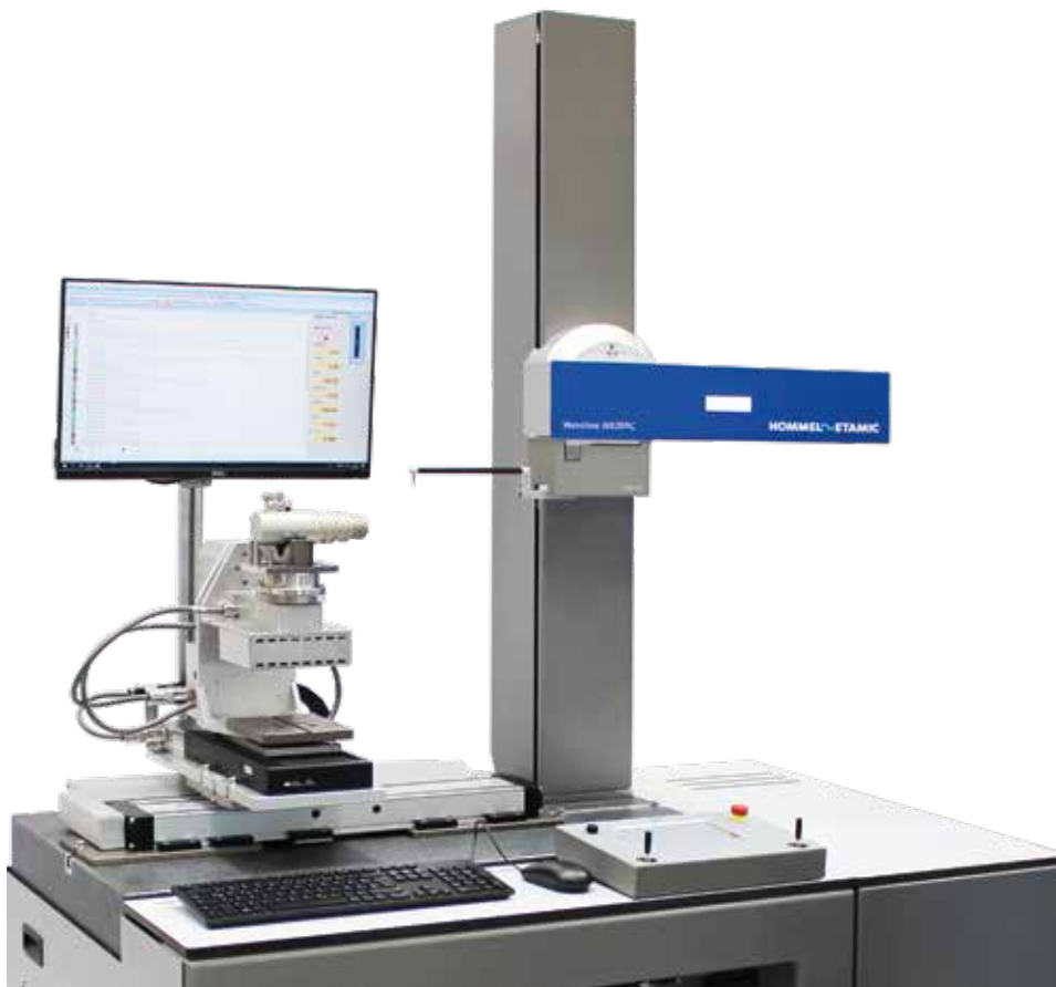
Waveline W820C measuring station with 800 mm column and Digiscan probe system for automated contour measurements
