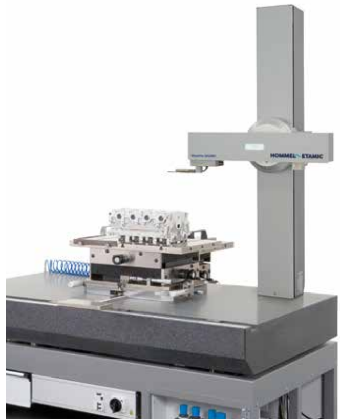
Waveslide measuring station with W920RC, 800 mm column, TKU400 probe system for roughness measurement and manually movable measuring table on air slides
